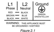
Should changing of the cord be necessary, gain access to the electrical connection terminal block and strain relief by removing the back panel (four screws).
